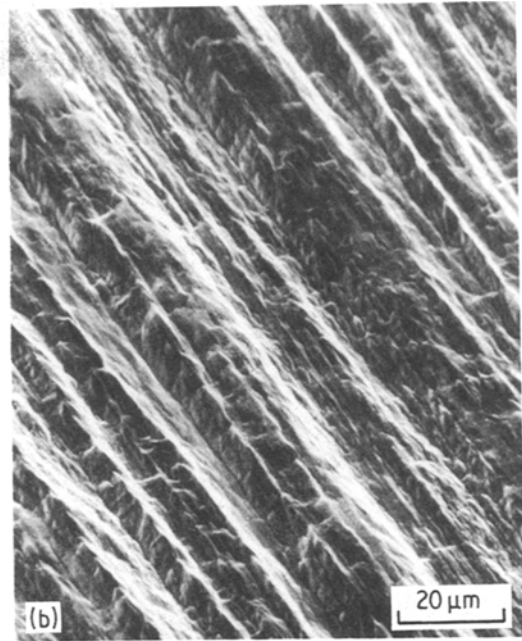
Figure 3 Surface topography of tantalum after ion sputtering at various angles of ion beam incidence, tilt about 0.8 rad. (a) Sample No. 11 at 0°; (b) sample No. 12 at 45° (~ 0.78 rad); (c) sample No. 13 at 60° (~ 1.05 rad); (d) sample No. 14 at 70° (~ 1.22 rad); (e) sample No. 15 at 80° (~ 1.4 rad).
