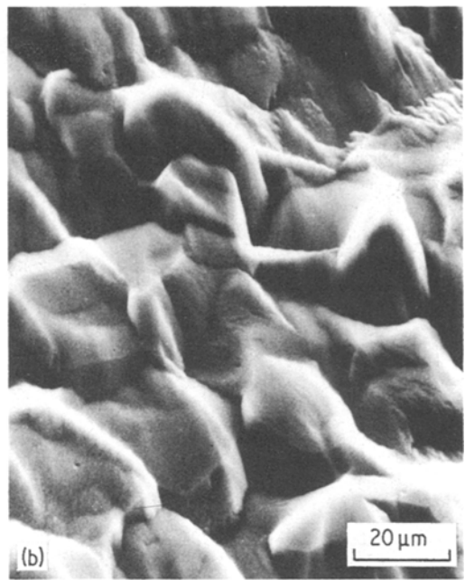
Figure 2 SEM images of titanium ion bombarded for 4 h at various incidence angles, tilt about 0.8 rad. (a) Sample No. 6 at 0°; (b) sample No. 7 at 45° (~0.78 rad); (c) sample No. 8 at 60° (~1.05 rad); (d) sample No. 9 at 70° (~1.22 rad); (e) sample No. 10 at 80° (~1.4 rad).
