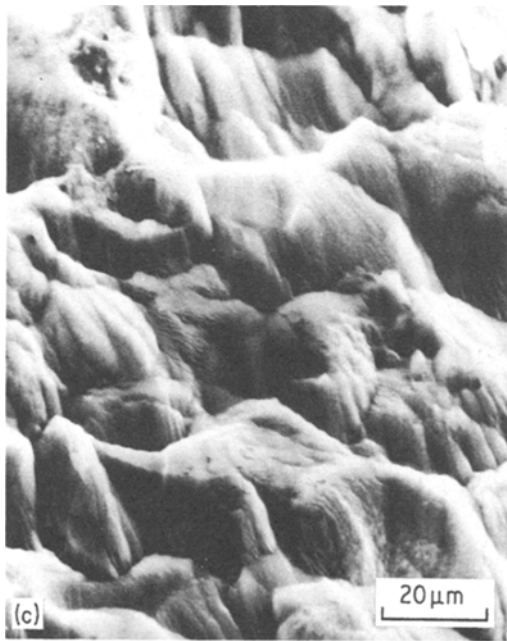
Figure 2 SEM images of titanium ion bombarded for 4 h at various incidence angles, tilt about 0.8 rad. (a) Sample No. 6 at 0°; (b) sample No. 7 at 45° (~0.78 rad); (c) sample No. 8 at 60° (~1.05 rad); (d) sample No. 9 at 70° (~1.22 rad); (e) sample No. 10 at 80° (~1.4 rad).
